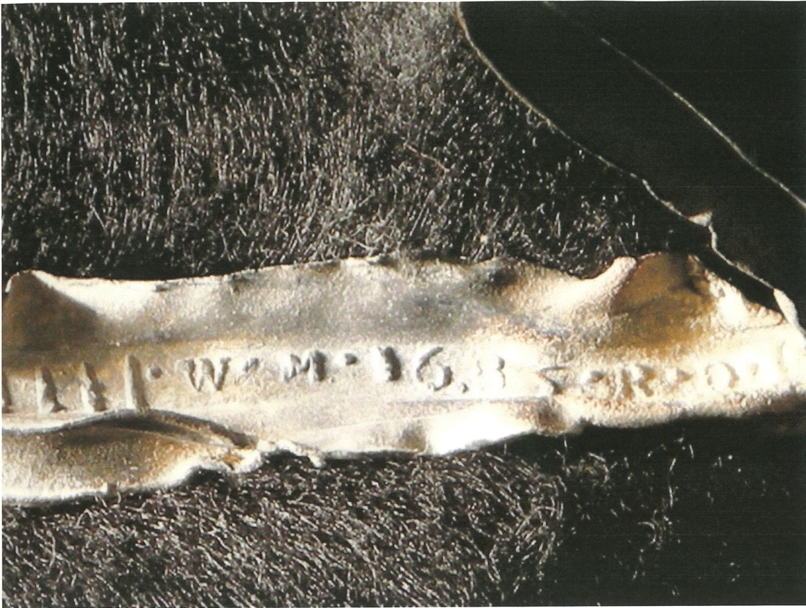
Figure 2. Detail of inscription in base of turned lead channel (·W·M·1685·R·D·).
